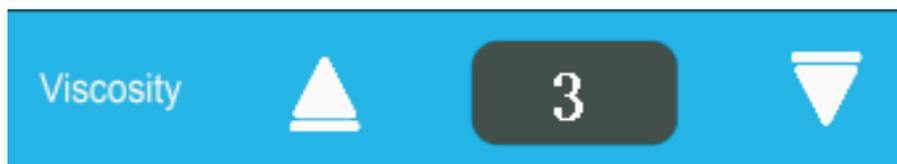
2. Viscosity Adjustment—modifies product viscosity level, from 1 – 8; viscosity rises with the level number.
